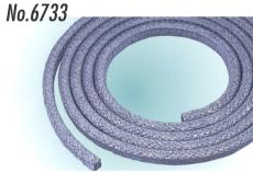
Pillar No.6733 is expanded graphite packing which is fabricated by braiding expanded graphite knitting varn reinforced with aramid fibers and treating it with a heat-resistant lubricant.
