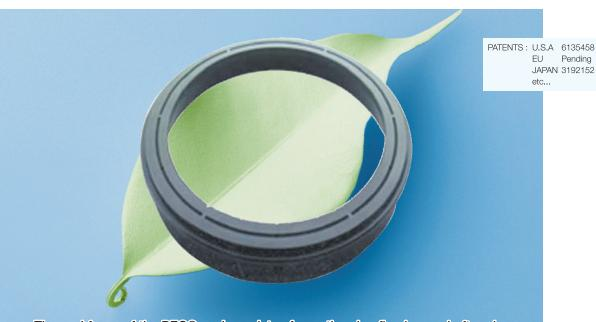
The seal faces of the PEC® seal consists of a mating ring fixed on a shaft and a seal ring which is movable axially in the casing. The seal ring has several orifices in the body and several debited shallow grooves on the seal face. Each of orifices and grooves is through-holed.
