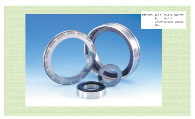
PILLAR Phoenix Seal series is a hydrodynamic gas seal with the special groove configurations for the dual-directionality. This groove pattern produces an efficient effect of dynamic pressure during rotation, which maintain optimum clearance between the seal faces in order to minimize the leakage.
